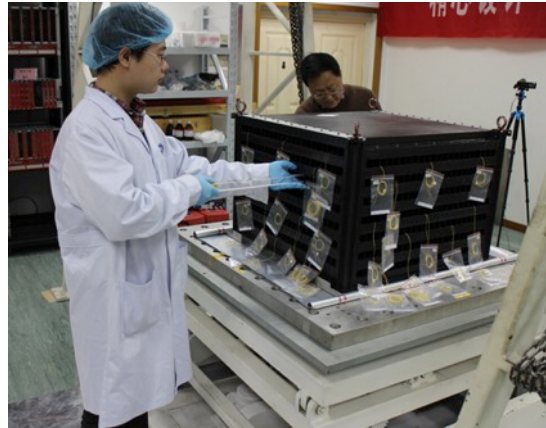
BGO crystal installation
